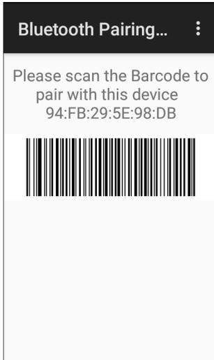
2. Using the RS507/RS507X or RS6000, scan the barcode on the screen.
