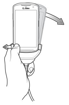
**2.** Push the Rugged Charge/USB Cable to the other side.
