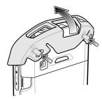
**4.** Insert the tab end of the hand strap into the slot on the device.
