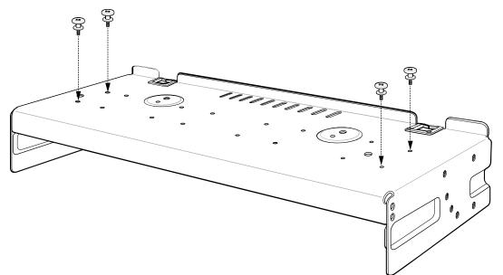
7. Align and install 5-Slot cradle onto studs of top tray.
