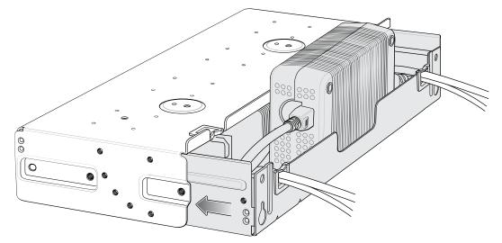
8. Install 16 M2.5 studs onto top tray as shown below.
