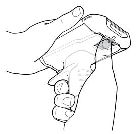
2. Slide the device forward and then rotate the bottom of the device up.
