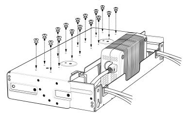
**9.** Align and install 4-Slot Battery Charger onto four studs.
