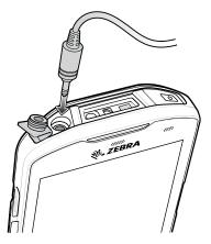
**3.** Connect the 3.5 mm connector plug of the headset into the 3.5 mm Audio Adapter.
