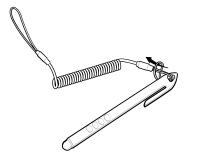
4. Insert the loop into the hand strap holder.
