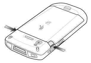
7. Lift the battery from the device.
