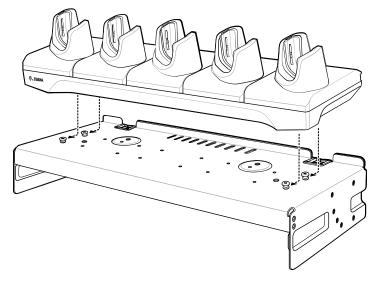
8. Secure cradle to top tray with two M2.5 safety screws. 9. Slide
