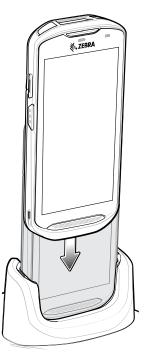
**2.** Ensure that the device is properly seated.
