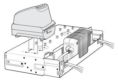
**10.** Connect DC Y cables to four 4-Slot Battery Chargers.
