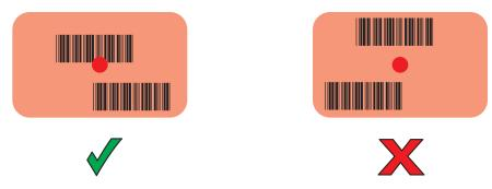
Pick List Mode with Multiple Barcodes in Aiming Pattern
