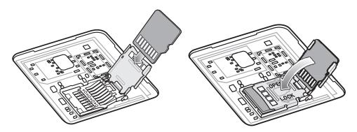
5. Close the microSD card holder and lock into position.
