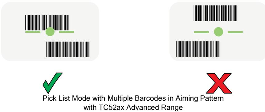
Pick List Mode with Multiple Barcodes in Aiming Pattern with TC52ax Advanced Range
