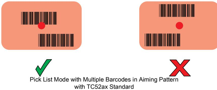
Pick List Mode with Multiple Barcodes in Aiming Pattern with TC52ax Standard
