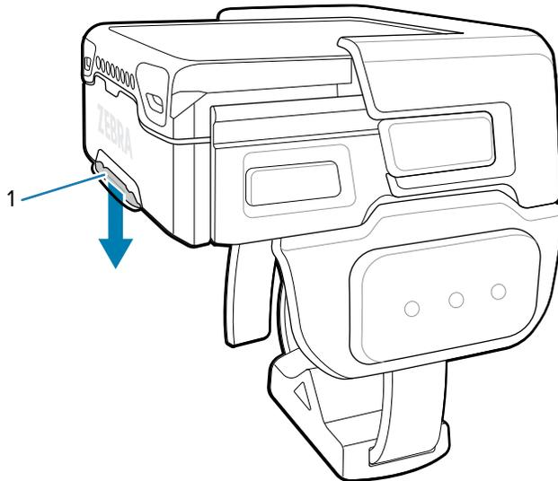
2. Slide the core (1) away from the trigger and shell assembly (2).
