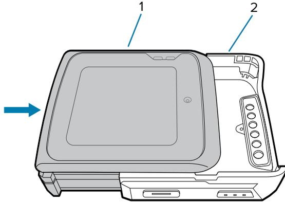
2. Insert the device, top first, into the wrist mount holder.
