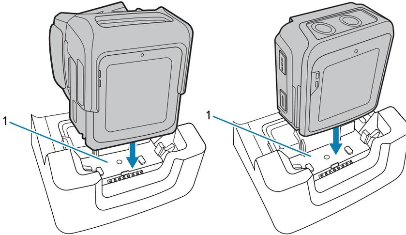
The device turns on and begins charging. The Notification LED on the touch panel shows amber while charging, then turns solid green when fully charged.
