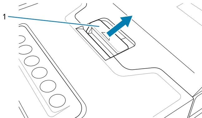
4. Lift the battery from the battery compartment.
