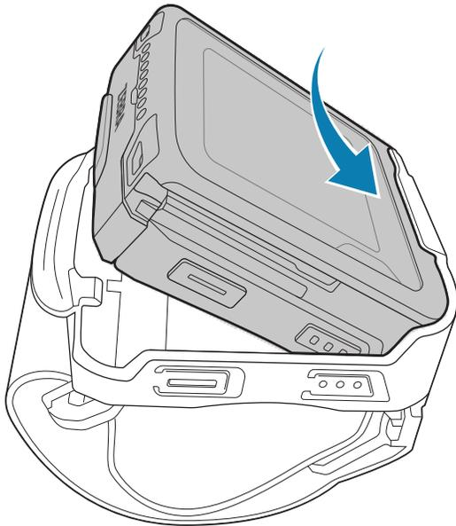
3. Press down on the wrist mount release tab (3) and the device simultaneously until the locking tabs (2) slide into the locking slots (1).
