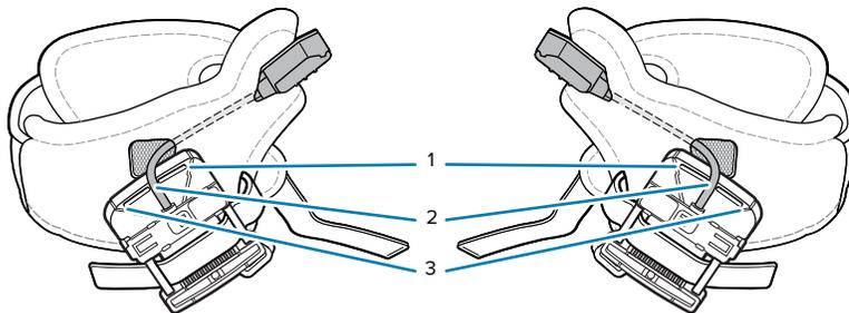
The BOH mount has three slots for the user to position the trigger cable. Insert the trigger cable into one of the slots according to the size of the user's hand:
