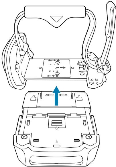
3. Rotate the trigger assembly so that the scan trigger is positioned next to the thumb.
