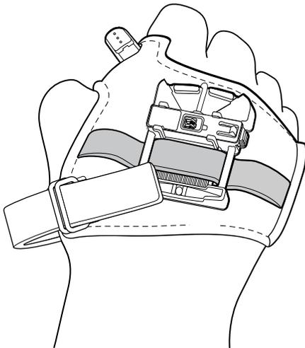
3. Slide the strap (1) through the buckle and secure the end of the strap in place with the hook and loop fastener.
