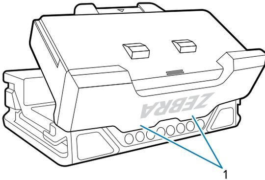
6. Press the battery down into the battery compartment until the battery release latches snap into place.
