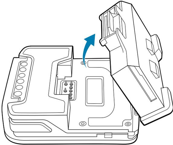
5. Align the battery so that the battery bottom engages the locking slots (1).
