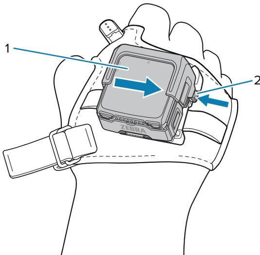
Release the button (2) when the device snaps into place on the BOH mount.
