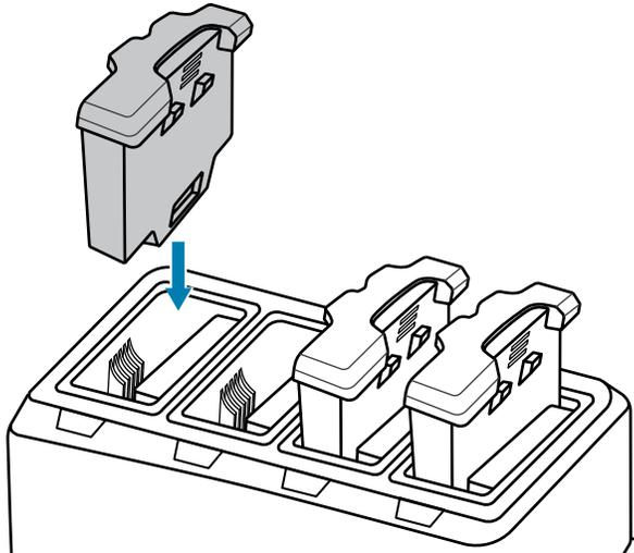
3. Gently press down on the battery to ensure proper contact.
