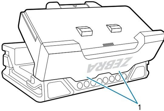
2. Press the battery down into the battery compartment until the battery release latches snap into place.
