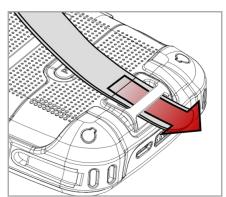
4. Pull the strap and attach the Velcro at the desired length.
