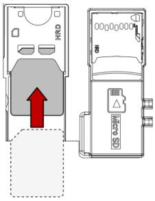
3. To remove the card, gently slide the card out from the slot.
