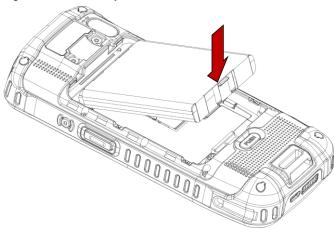
5. Engage the battery cover from the top, and then press the edge of the cover to close it firmly. Figure 10 Close battery cover
