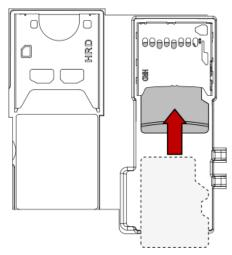
4. To remove the card, gently slide the card out from the slot.
