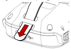
4. Slide the strap through the buckle and latch the buckle at the appropriate length.
