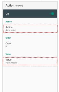
6. "Point Mobile" string will be added to decoded CODE128 data.
