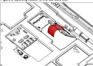
3. Slide the card into the slot with the contacts facing down.
