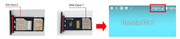
(A) Put in two SIM Cards or (B) Put in one SIM Card and an SD Card.
