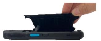
3. Align the battery with the bottom slot in the battery compartment.
