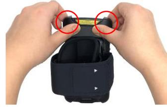
2. Use your thumbs and push the EA520 terminal on its yellow part, until the terminal completely detaches from the boot case.
