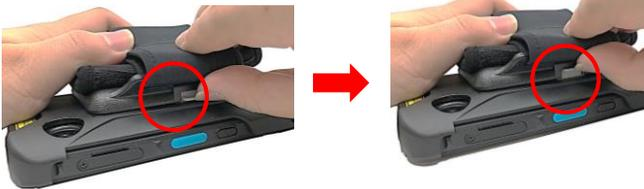
2. Keep holding the button and pull the wearable kit toward the direction of your chest to remove.
