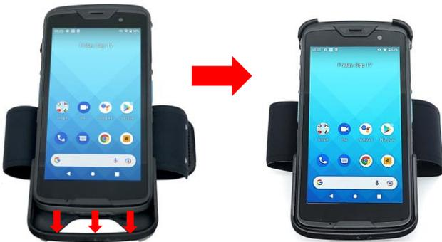
**Note:** You can use the single slot USB/charging cradle or USB Type-C cable without removing the wearable kit after removing the detachable part on the single slot cradle
