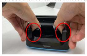
Use your thumb to lift up to take out the detachable part. Once it got unhooked, you can lift it up from both sides.
