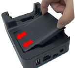
2. Press down the battery while holding the buckles, then release after the battery is completely insert into the battery compartment.
