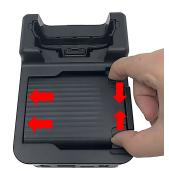
2. Lift the battery while holding the buckles to remove.
